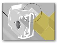
7. If curved, fit the centre position of the track. Then fix head rail end by fitting screws through track stops.
