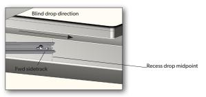
4. With both side tracks fitted and the handle pointing downwards feed the whole blind into the side tracks taking care to keep the cords outside the gliders. Keep the blind together.
