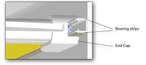
5. Lift the blind and side tracks up so that you can fit the head rail into the head rail clips.
