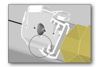
Now push the head rail back until the clip lock over the rib on the back of the head rail.
