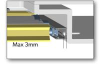
10. Operate the blind, opening and closing a few times. There should be enough tension to allow the moving rail to be left in any position and it will stay there. The gliders should run smoothly in the side tracks.
