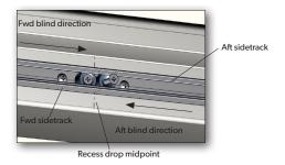
9. Fit the remaining screw in the side tracks, be sure not to damage extrusion or paintwork to ensure smooth travel of guides
