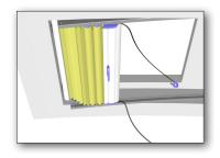
6. Clip the head rail into the head rail clips by hooking the front of the rail into the clip and then pushing back until the back hook clips over the lip on the head rail (the head rail and the fabric have been sectioned in this view to show the clip more clearly).
