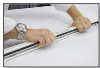
Fitting opposite headrail for single ended assemblies as per steps 9a & b.
