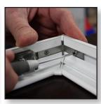
3. Assemble corners as shown to **one end only**, ensure profile is tight to mitre corner.
