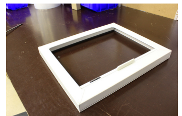
23 Test blind by deploying and stowing two or three times to ensure blind operates correctly.
