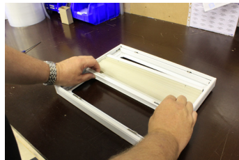
19 Turn frame round to prepare to fit headrail.
