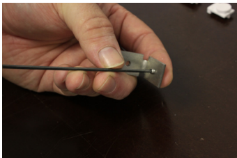
2 Pre load grub screws in to brackets.
