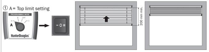
Blind must be down at least 200 mm before setting top limit. Press I or II and hold until the blind stops by itself.
