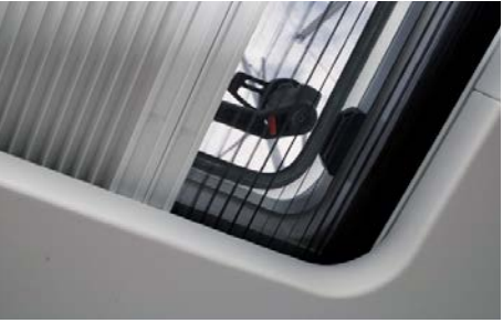
5. Natural ventilation Flyscreen lets air into the cabin for a fresher interior.
